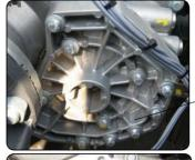
1) Remove the gearbox cover and make sure that the parts belonging to the oil lube pump are well located in their seats.
