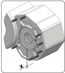
5) Keep the ring pressed into its seat and check the value between gearbox surface and ring surface ( value  ${\bf X}$  ).
